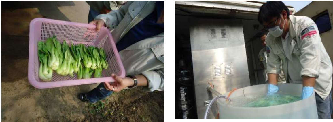
Figure 14 Pak chai washing with ozonated water, which was assigned the concentration of more than 0.6 ml/l
